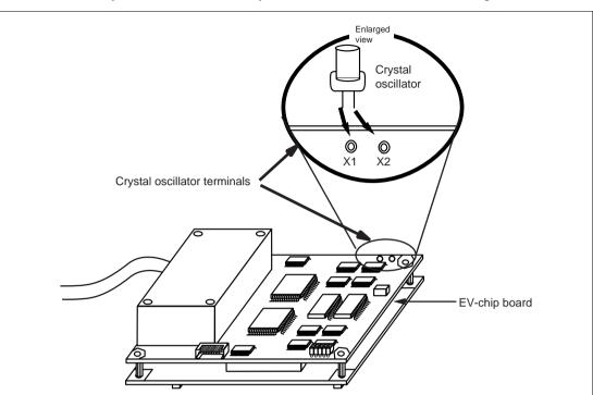
— To use the crystal oscillator mounted on the EV-chip board Install a crystal oscillator into the crystal oscillator terminals on the EV-chip board.
